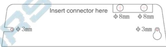
Apply the mounting template to drill holes
